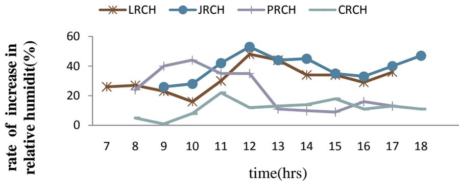
Figure 10: Periodic rate of increase in relative humidity at 4.0 m/s for the four cooling pads
