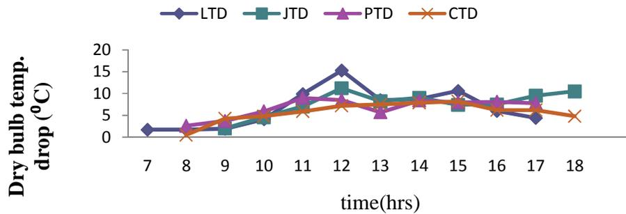
Figure 7: Periodic drop in Temperatures at 4.0 m/s for the four cooling pads
