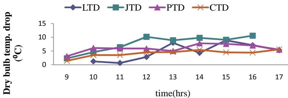
Figure 6: Periodic drop in Temperatures at 3 m/s for the four cooling pads
