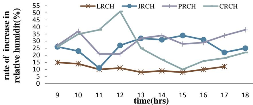
Figure 11: Periodic rate of increase in relative humidity at 4.5 m/s for the four cooling pads
