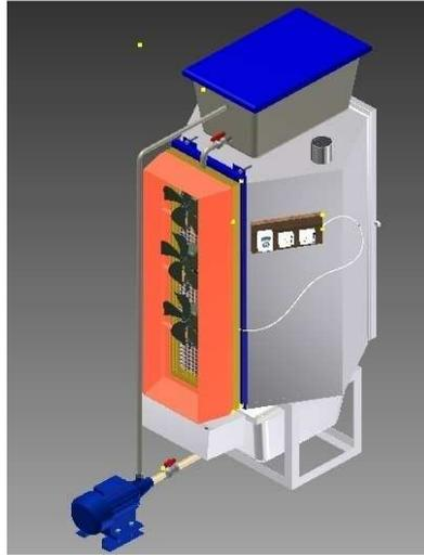
**Figure.5: schematic active evaporative cooling system**
