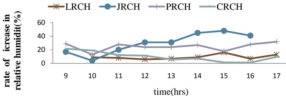
Figure 9: Periodic rate of increase in relative humidity at 3 m/s for the four cooling pads
