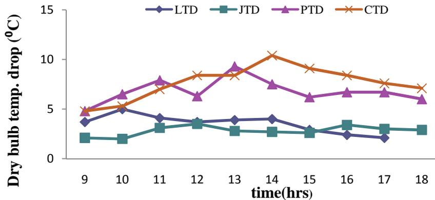
Figure 8: Periodic drop in Temperatures at 4.5 m/s for the four cooling pads
